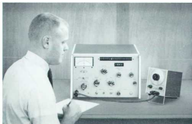
Fig. 1. New -hp- Model 310A Wave Analyzer measures amplitude of individual frequency components in 1 kc-1.5 Mc region over a dynamic range of more than 75 db. SSB carrier system testing in this frequency range is facilitated by carrier reinsertion provision contained in analyzer.
