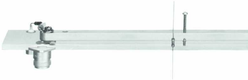
Fig. 8. Broadband stripline circuit used in bench work with Step Recovery Diode. Either glass or ceramic style diodes can be accommodated as shown.
