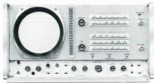
Fig. 3. Controls needed for complete manual control of oscilloscope are available behind flip-down cover. Only those controls necessary for readout of programmed ranges and for manual search for signal, when in programmed operation, remain exposed when cover is closed.
