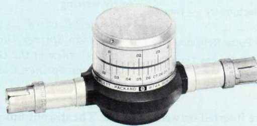
Fig. 2. -hp- Model 874A Calibrated Susceptance simplifies TDR measurements of small reactive discontinuities. Susceptance provides basis for comparison measurements of capacitive discontinuities from 0 to 1 pF and inductive discontinuities from 0 to 2.5 nH.
