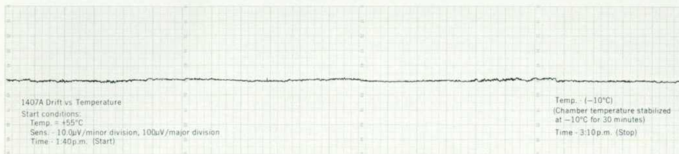
Fig. 3. Strip chart recording shows insensitivity of plug-in stabilized dc level to variations in temperature. At start of recording scope was in environmental chamber at 55°C. Chamber temperature was reduced to -10°C over period of 1 hour and then held at that temperature for remaining 1/2 hour of test. Trace deviates less than \pm 20 \mu\text{V} during test.
