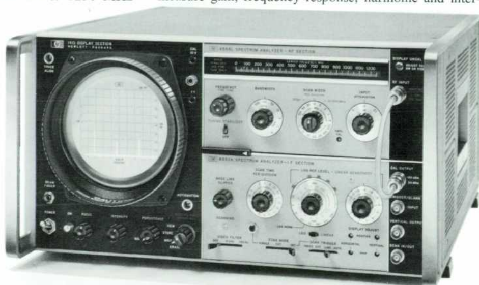
Fig. 1. A new plug-in RF section makes this a 0.5-to-1250-MHz spectrum analyzer—or frequency-domain oscilloscope, if you prefer. It has absolute amplitude calibration, automatic phase lock, and simple controls. Its frequency response is flat within \pm 1 dB from 1 to 1000 MHz. It has a 60 dB spurious free display range, -120 dBm maximum sensitivity, and scan widths from 20 kHz to 1250 MHz. Variable-persistence and large-screen displays are optional.
