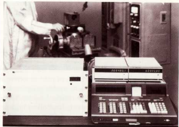
On top of the calculator are two 10783A Numeric Displays. At left is the 10740A Coupler.
