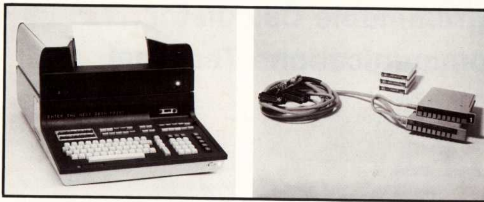
Fig. 1. Model 11284A Modem and Autodialer Interface and three plug-in data communications ROMs convert Model 9830A Calculator to a data communications terminal. Depending on the ROMs installed, the calculator can act as a timesharing terminal or as a remote batch terminal.
