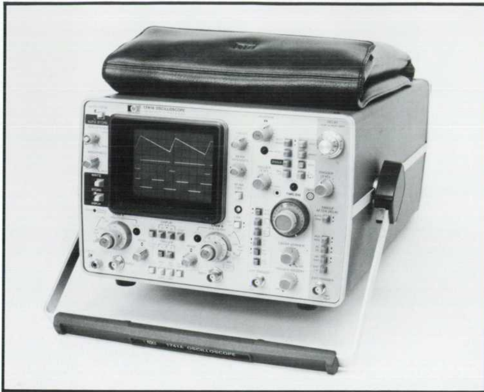
Fig. 4. New Model 1741A Oscilloscope has variable persistence and storage modes of operation in addition to having all the other attributes of a high-quality, laboratory grade, 100-MHz Oscilloscope. Storage controls, with LED indicators to show what state the instrument is in, are grouped conveniently to the left of the CRT.
