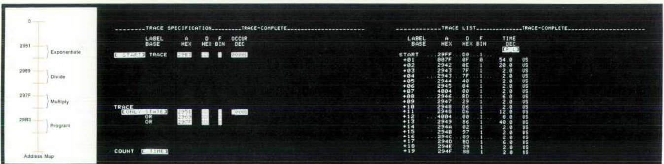
Fig. 14. Selective trace can be used to trace program flow between major program segments and the order in which subroutines are called following initiation of program execution at address 29B3. The COUNT feature discloses how much time is spent in each subroutine.
