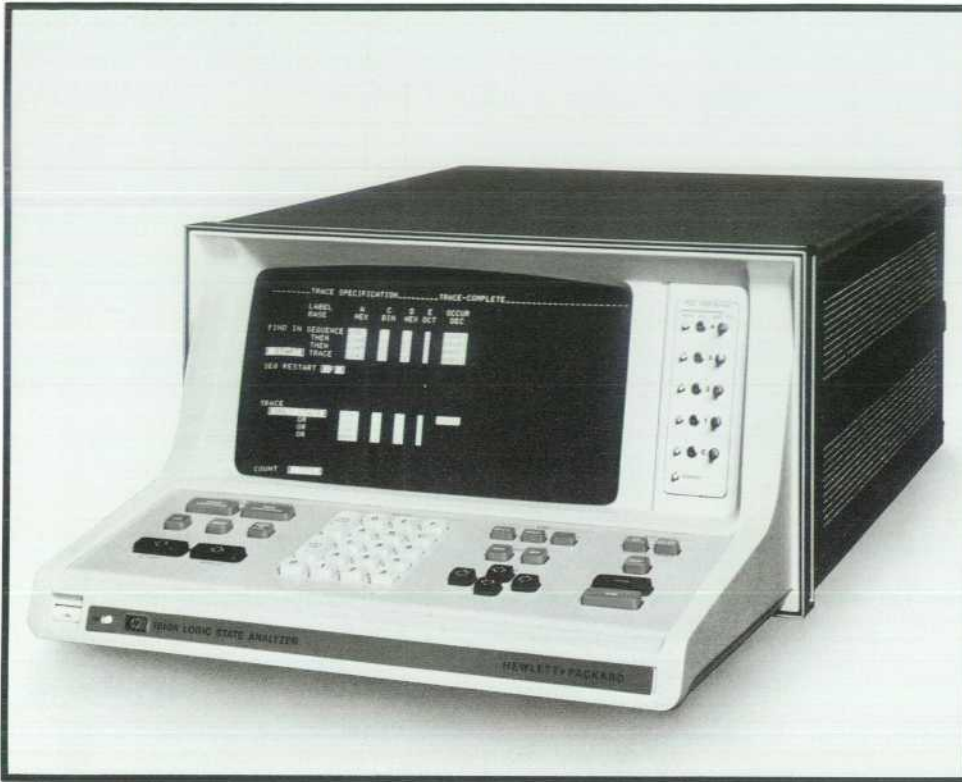
Fig. 1. Model 1610A Logic State Analyzer traces the flow of states up to 32 bits wide in minicomputers, microprocessor-based systems, and other sophisticated logic systems. The interactive display and keyboard simplify the establishment of highly selective protocol for capturing only the data of interest.
