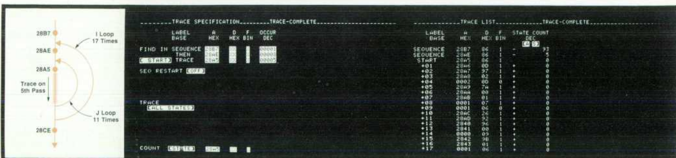
Fig. 10. Any pass in a loop nested within other loops can be captured for display by using the OCCURRENCE feature in conjunction with sequential triggering. In this example, tracing begins with the eighth pass of the J loop during the fifth pass of the I loop.
