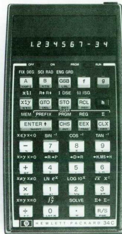
Fig. 1. The HP-34C, a new handheld programmable calculator, has two keys that are new to handheld calculators— ∫ (integrate) and SOLVE , a numerical equation solver, is described in this article.
