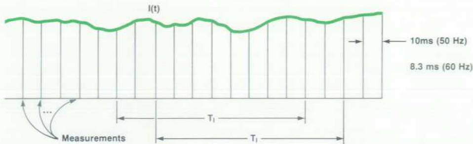
Fig. 2. Measurement fluctuations are smoothed by digitally averaging several readings. As each new measurement value is added, the oldest value is subtracted to maintain a running average.
