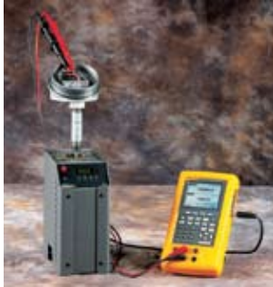
Hart Scientific dry-wells interface directly to the Fluke 744 for fully automated calibration.
