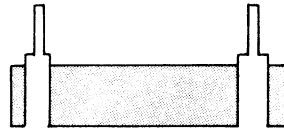
Example of (+) synchronizing signal
