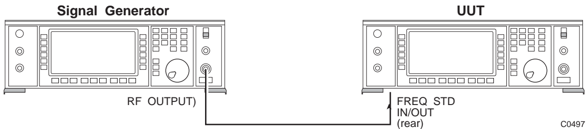
Fig. A-25 Frequency standard locking test set-up
