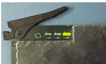
Fig. 2-13 Dithering LED Status Indicator
