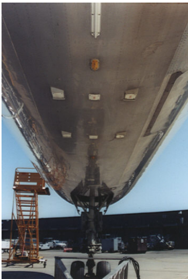
Fig. 1-8 Triple LRRR Antenna Installation (ARINC square patch type)
