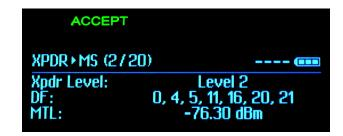
The 20-character 4-line display provides for easily viewable data and parametric measurements as required for Mode S Elementary and Enhanced Surveillance testing. For legacy test modes, the menu structure and displayed data format have been retained so that minimal changes are required of fielded procedures.
