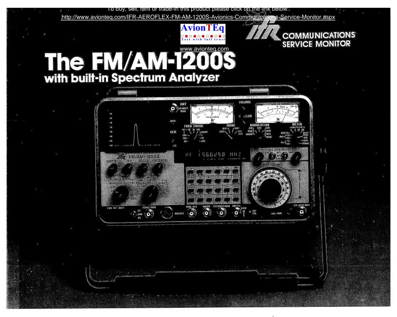
The FM/AM-1200S and FM/AM-1200A are multi-function, microprocessor controlled Communications Service Monitors designed to meet the requirements of most radio maintenance applications throughout the RF frequency range of 250 kHz to 1 GHz. Fully portable, both monitors deliver features and special functions never before available with any service monitor in their price range.
