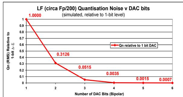
Figure 5. Effect of ADC/DAC resolution on noise.
