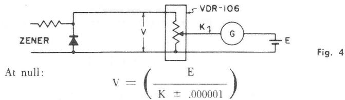
Where K is the dial setting. The uncertainty to which E is known must be allowed for, also. It is interesting to note that, with a primary standard cell set, such as the SCO-106 illustrated below, and a value of V near 6 volts, the absolute accuracy of measurement is about 0.0003%.
