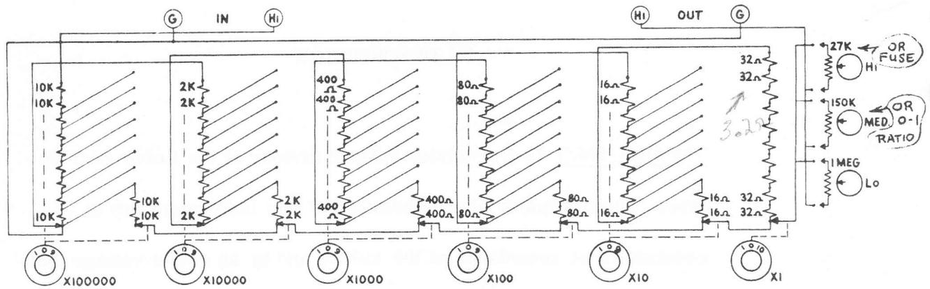
The VDR-106 is an older version of this divider with six decade dials and no Ratio switch. In place of the Ratio switch is a "medium sensitivity" key which inserts a 150 kohm resistor in the output circuit. Some of these dividers have a 27K resistor in place of the 1/100th amp instrument fuse. All older models can be modified to conform to the specs for the VDR-106/7.
