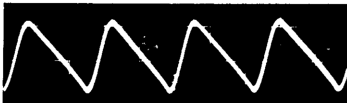
FIGURE 10. Wave Form at Junction of Diodes D301 and D302 (Figure 27). Vertical setting is 1 volt/cm; horizontal, 2 milliseconds/cm. Output is approximately +400 volts dc.
