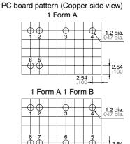
The above shows 2 coil latching type. No.2 and 5 terminal are eliminated on single side stable type.
