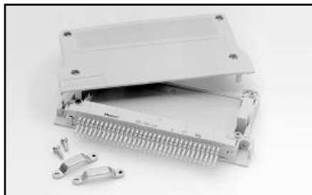
Model 7011-KIT-R: 96-pin female DIN connector with solder eyelets and strain relief. This kit can be used for assembly of custom cables to connect with the connectors on the 7011-C, 7012-C, 7013-C, 7015-C, and 7018-C switch cards. Also connects with the 7011-MTR bulkhead mount male connector. For use with: 7011-C, 7012-C, 7013-C, 7015-C, 7018-C
