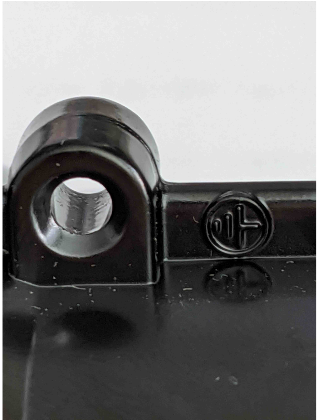
fan unthreaded grounding hole.jpg (139.15 kB, 3024x4032 - viewed 58 times.)
