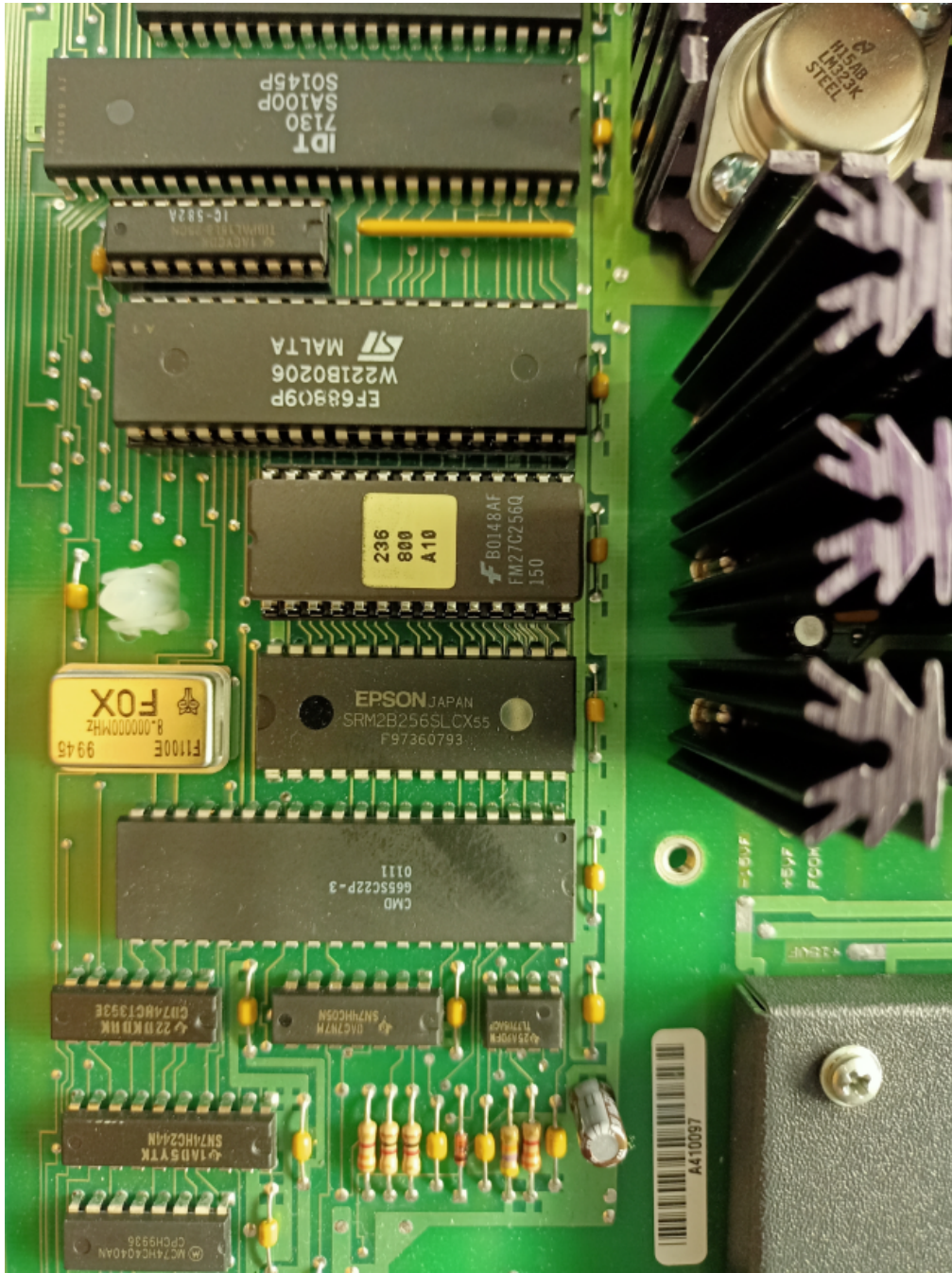
On the mainboard there is a second device which is also marked with a firmware version (236 801 A10). But I don't know if you also need it. Is an EEPROM ev. are there only the calibration data stored.
