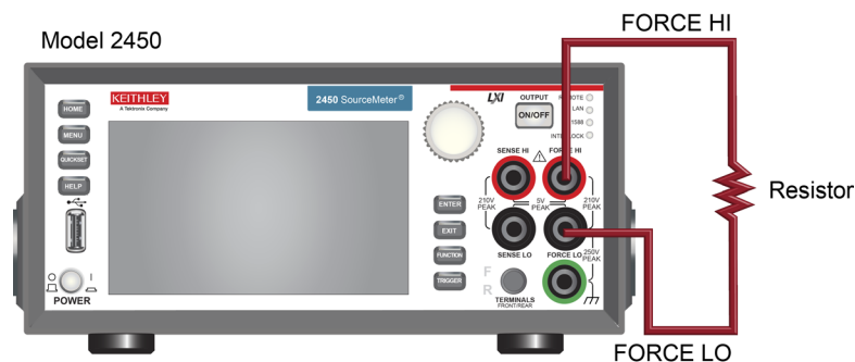
Figure 16: Model 2450 2-wire front-panel connections
