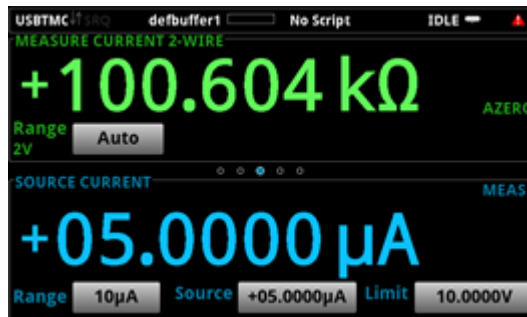
Figure 61: Resistance measurement SIMV SCPI example
