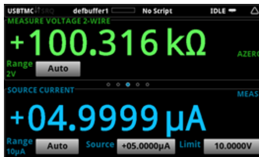
Figure 62: Resistance measurement SIMV and read ohms
