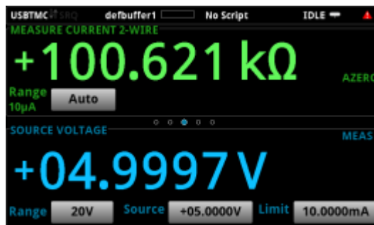
Figure 59: Resistance measurement using SVMI and reading ohms
