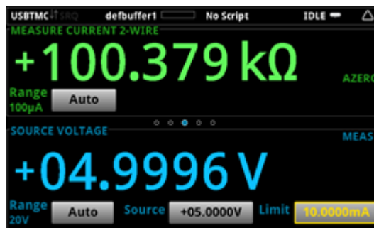
Figure 60: Resistance measurement SVMI and reading ohms
