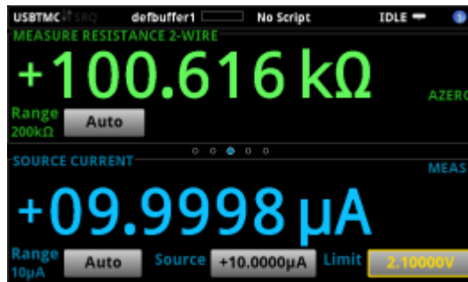
Figure 63: Resistance measurement using resistance function
