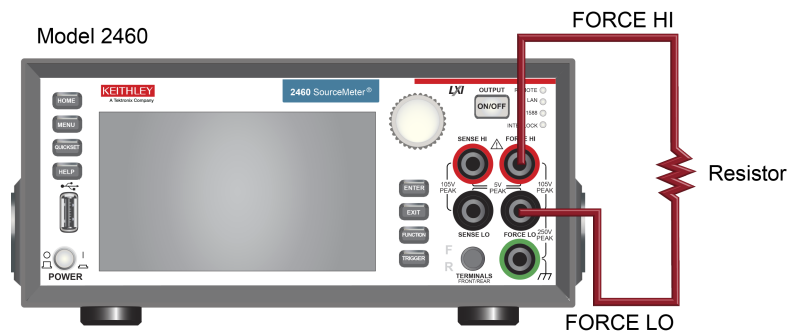
Figure 17: Model 2460 2-wire front-panel connections
