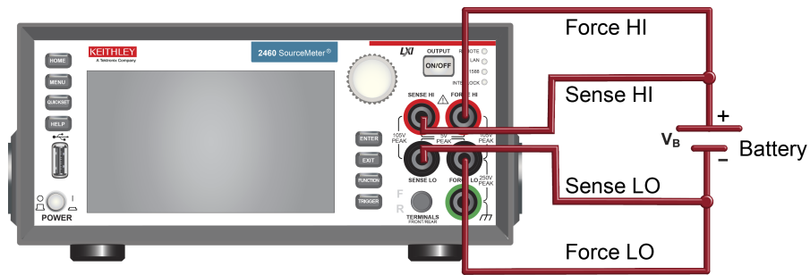
Figure 28: Front-panel connections for the battery discharge-charge application
