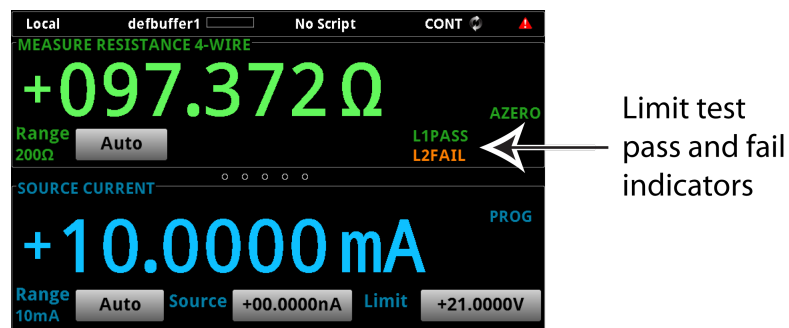
Figure 109: Limit test front panel indicators
