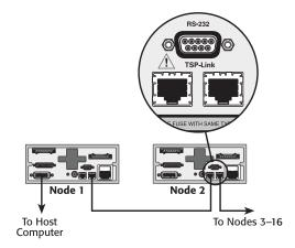
Each SourceMeter has two TSP-Link connectors to facilitate chaining instruments together.
