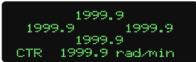
Figure 2-18. An Absolute Rate Measurement With Air Density Corrections and the Front Panel Gain Factors Disabled
