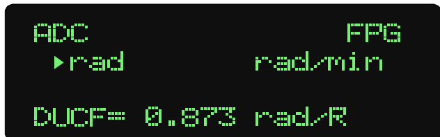
Figure 2-11. The Units Select Screen with Dose Measurement Units Selected
