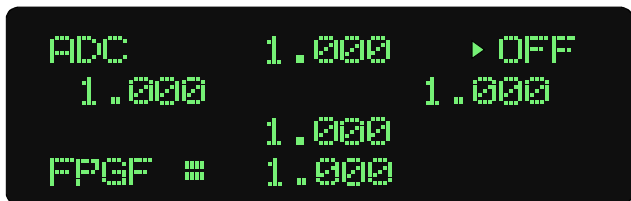
Figure 2-15. The Gain Select Screen With the Front Panel Gain Disabled
