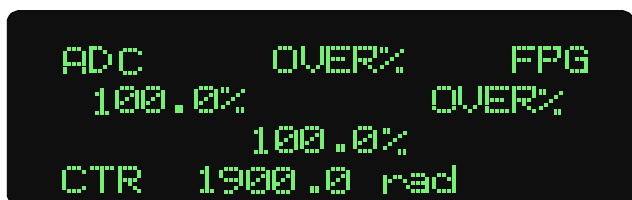
Figure 2-23. Overranging the Top and Night Channels of the Electrometer
