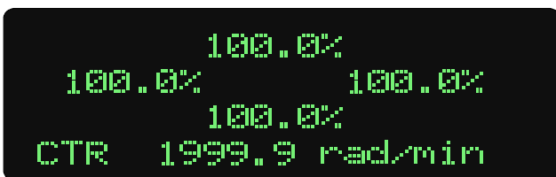
Figure 2-21. A percentage rate measurement with both air density corrections and the front panel gain factor disabled
