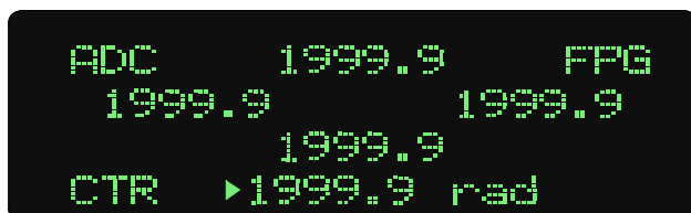
Figure 2-26. An Absolute Dose Measurement With the Center Ion Chamber Selected for FPGF Modification
