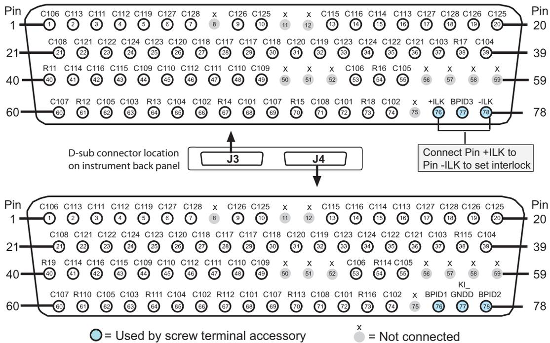
**Pin assignments and signal naming: Single 16x28 configuration**
