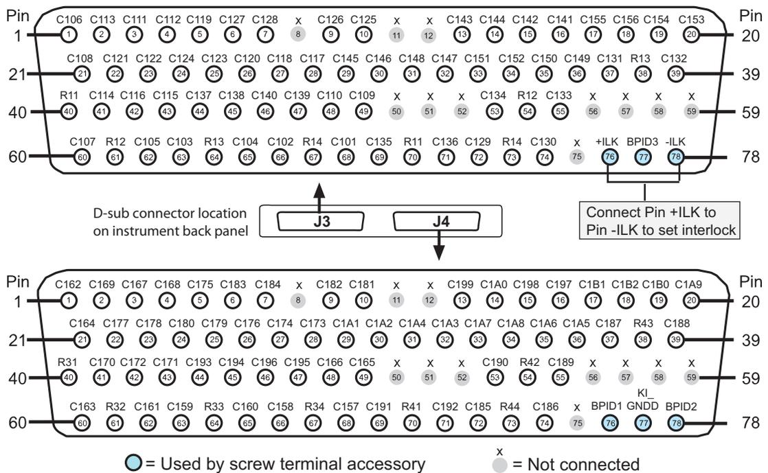
**Pin assignments and signal naming: Single 4x112 configuration**
