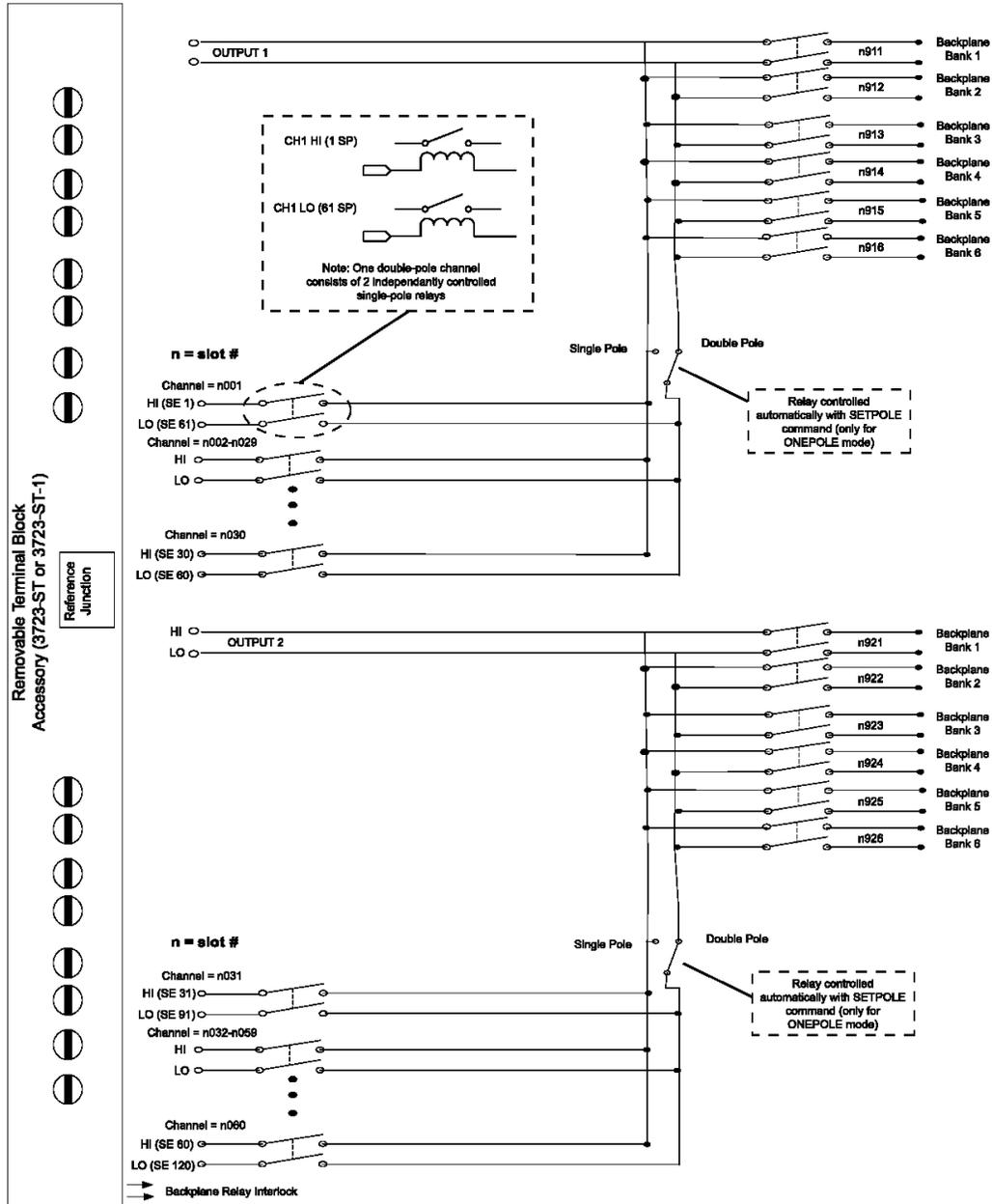
The following figure provides a switching schematic for the Model 3723 in single-pole mode.
