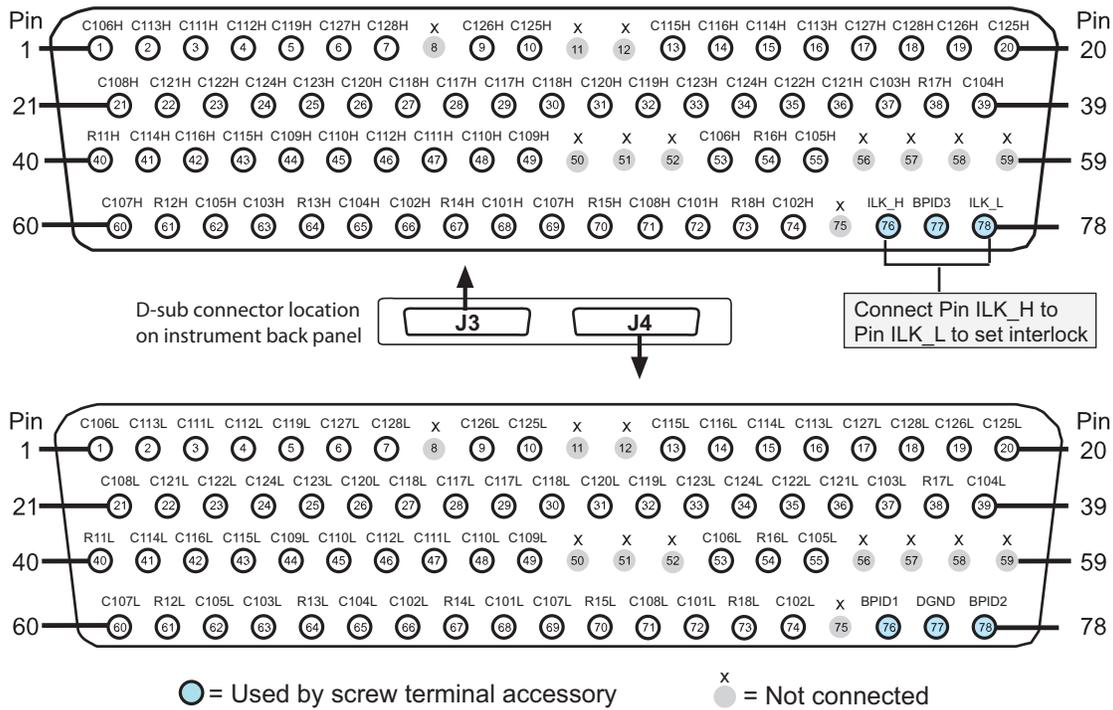
**Pin assignments and signal naming: Single 8x28 2-pole configuration**
