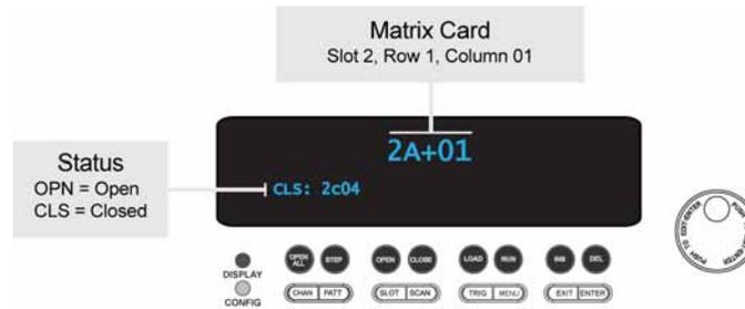
**Figure 39: Model 3732 matrix card display slot 6**
