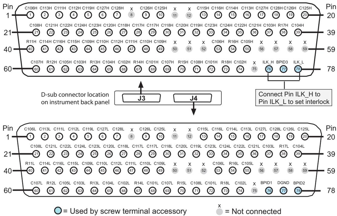
**Pin assignments and signal naming: Single 4x56 2-pole configuration**
