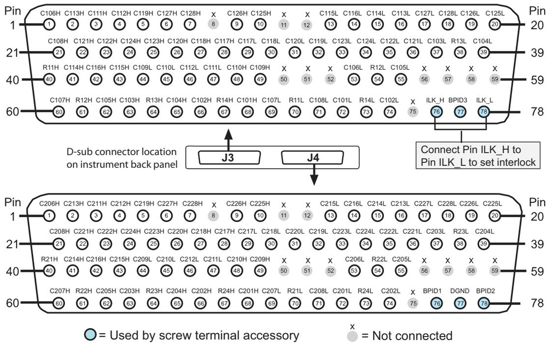
**Pin assignments and signal naming: Dual 4x28 2-pole configuration**
