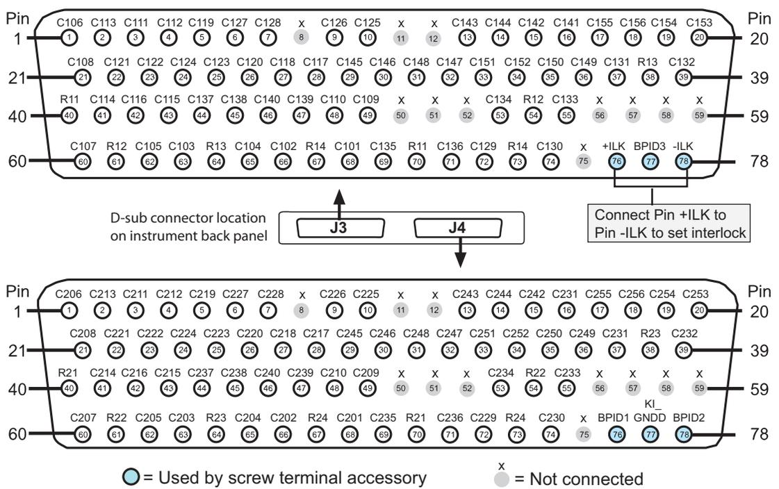
**Pin assignments and signal naming: Dual 4x56 configuration**
