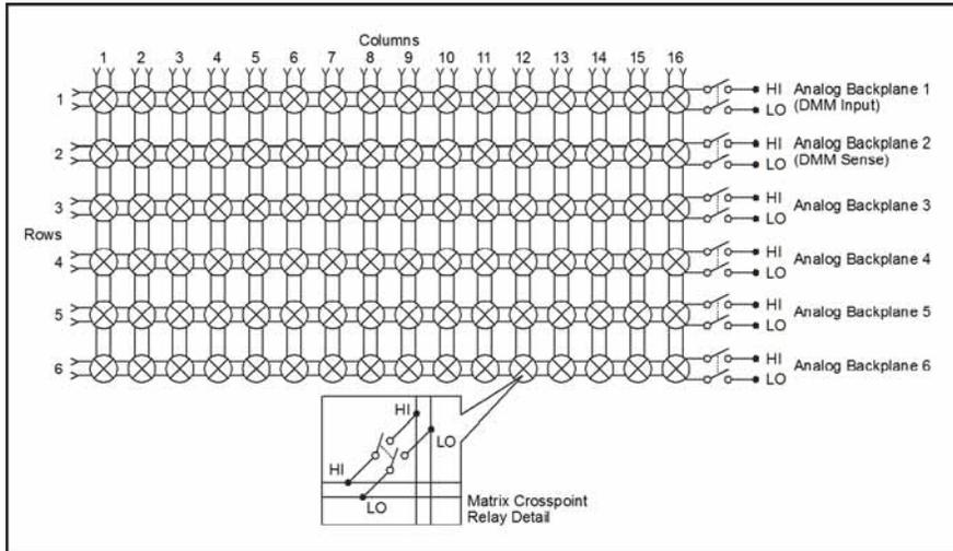
The channels on the Model 3730 are matrix channels. Unlike multiplexer (MUX) channels, matrix channels do not have a DMM configuration associated with them. Therefore, specifying a matrix channel in the channel list parameter to the `dmm.setconfig()` function generates an error. To connect a DMM configuration to matrix channels, create a channel pattern with desired channels and analog backplane relays.
