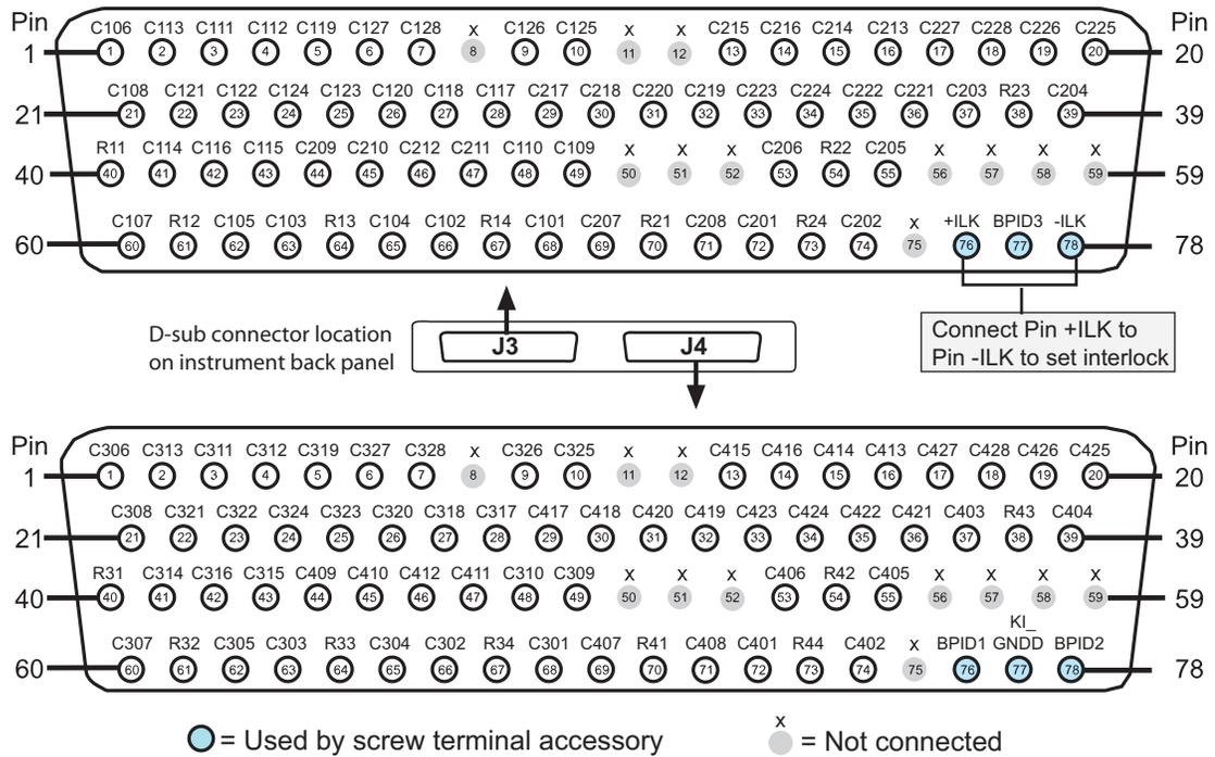
**Pin assignments and signal naming: Quad 4x28 configuration**
