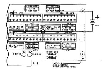
Figure 3. Typical AIM3 Differential Connections (Channel 0 shown)
