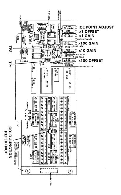
Figure 4. AIM3 Calibration Adjustmets
