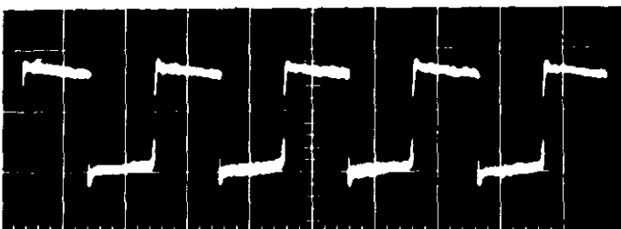
FIGURE 13 (left). Correct Waveform at Junctions of Diodes D101 and D102. Vertical sensitivity is 1 volt/cm; horizontal sweep is 5 milliseconds/cm.
