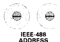
Figure 4-11 Rear panel - IEEE-488 address switches
