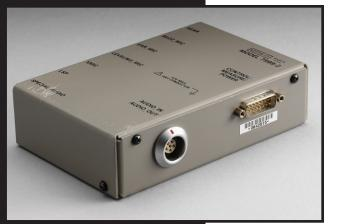
The 7999-2 Three-Pole Audio Multiplexer Module contains a three-pole 1×3 multiplexer, and a 3-pole 1×4 multiplexer for switching audio signals. For minimizing the effects of noise, the input and output connectors are shielded, high quality audio connectors, and the module is enclosed in an aluminum case. In addition, each input and output line has an RF filter for filtering out high frequency noise.
