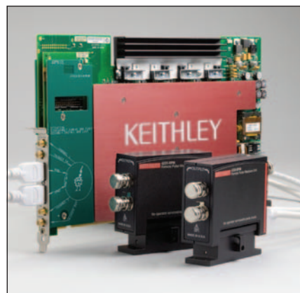
Figure 7. Model 4225-PMU Ultra-Fast I-V Module and two Model 4225-RPM Remote Amplifier/Switches, available for the Keithley Model 4200-SCS characterization system.
