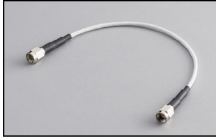
CA-452A: 20.4cm (8 in) RG188 coax cable terminated with an SMA male plug on each end, 50Ω impedance.
