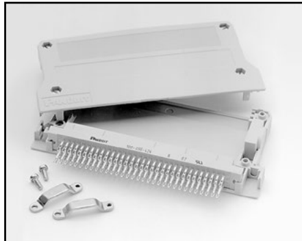
Model 7011-KIT-R: 96-pin female DIN connector with solder eyelets and strain relief. This kit can be used for assembly of custom cables to connect with the connectors on the 7011-C, 7012-C, 7013-C, 7015-C, and 7018-C switch cards. Also connects with the 7011-MTR bulk-head mount male connector.
