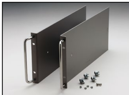
Model 7002-RMK-1 Fixed Rack Mount Kit: Two 7 in. flanged brackets and hardware for mounting the Model 7002 in a standard 48.3cm (19 in) equipment cabinet. Can be used with Models 8000, 8000-10, 8000-14, or 8000-17.
