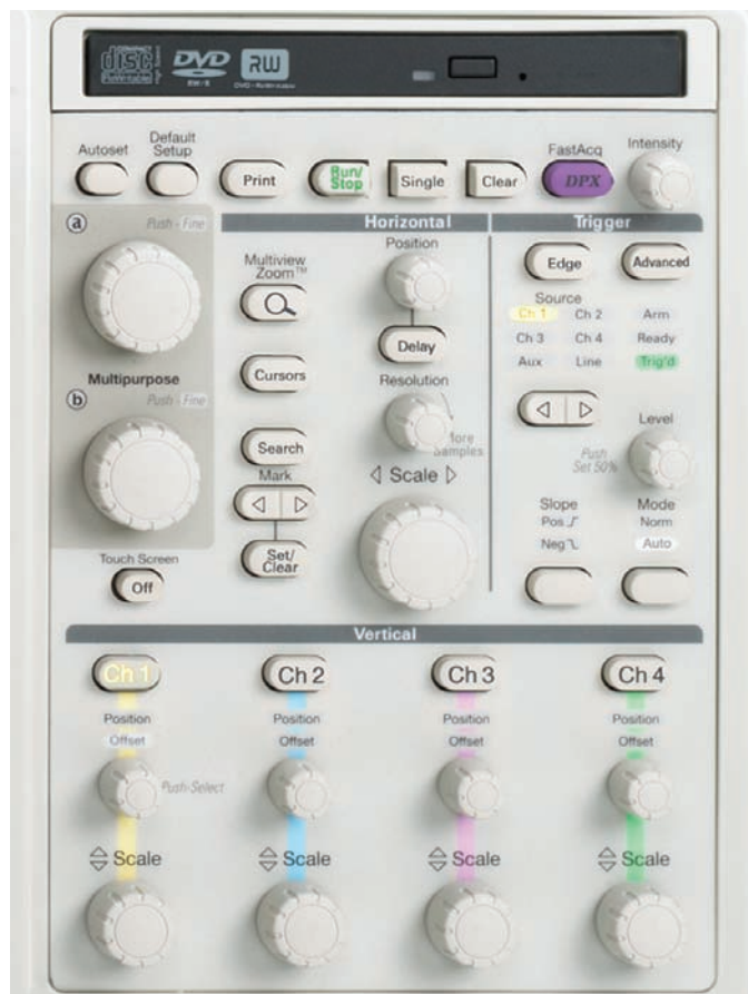
Figure 20. Front-panel control section of an oscilloscope.
