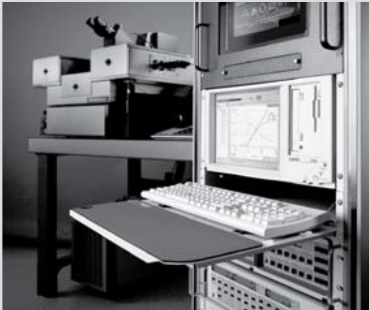
Figure 4. Example of a Windows®-based semiconductor characterization system, the Keithley Model 4200-SCS.
