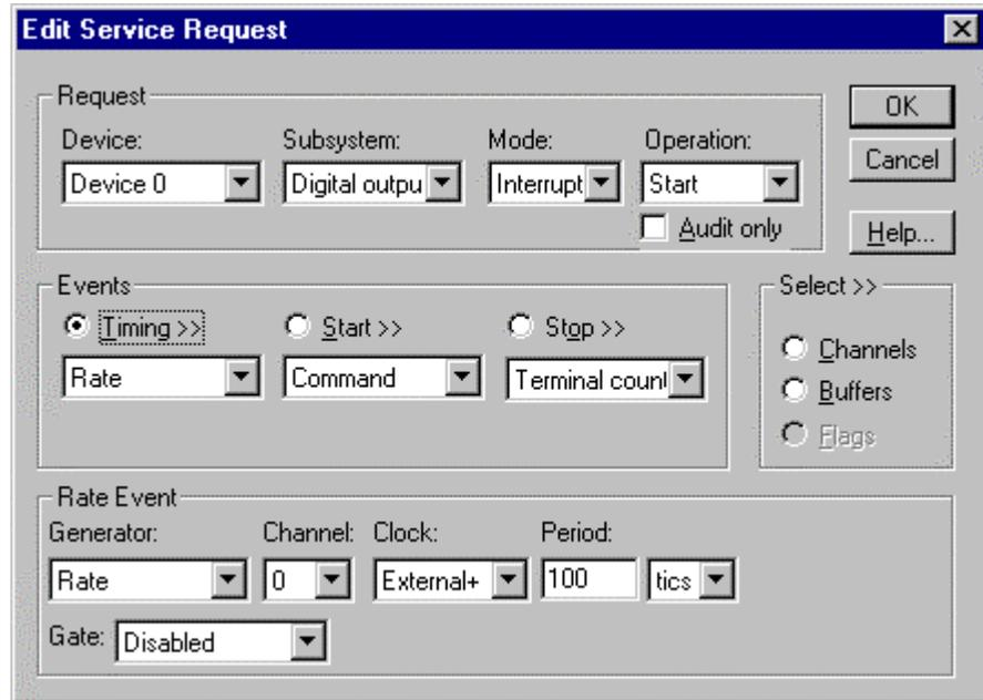
How to set up the KPCI-PIO24 for fixed rate sampling using an external clock.
