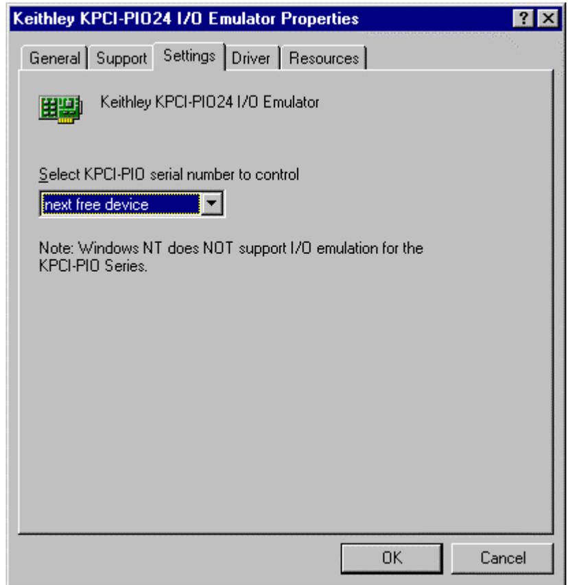
3. To assign the driver's I/O address to a specific KPCI-PIO board, select the board's serial number in the drop-down list. Note that this list only displays currently installed boards.
