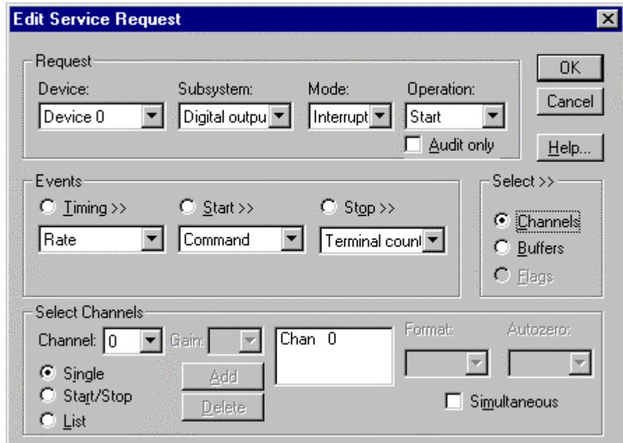
*How to set up the KPCI-PIO to write from a single channel*
