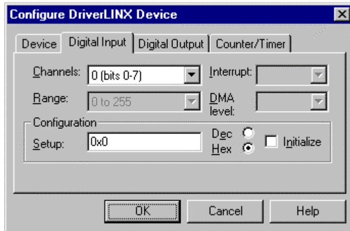
Use the Digital Input Subsystem page to tell DriverLINX the Configuration Setup of the KPCI-PIO's digital input/output channels. You can also use this page to view the Channel number and Range of each digital input channel.
