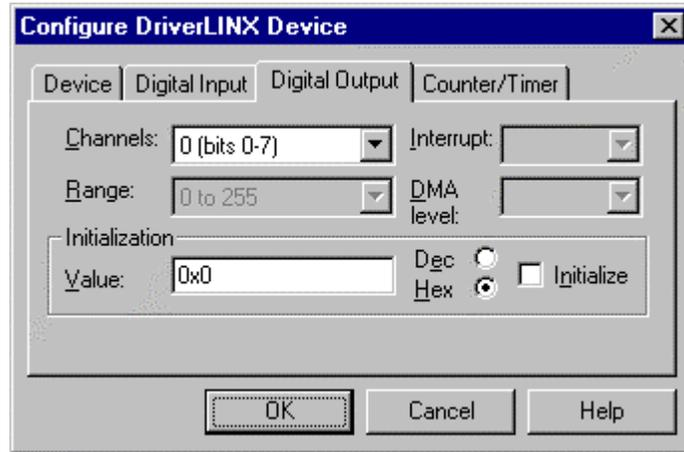
Use the Digital Output subsystem page to change the default digital output port initialization values.
