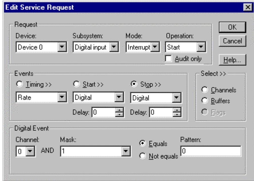
*How to set up the KPCI-PIO for pre-triggered digital input.*
