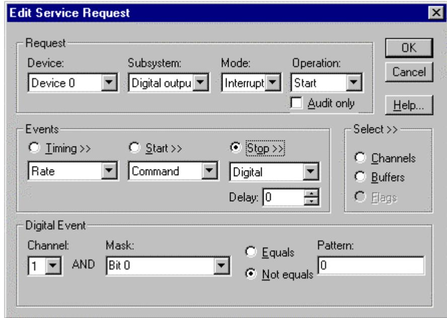
How to set up the KPCI-PIO for pre-triggered digital output.
