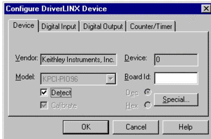
Use the Device Subsystem page to tell DriverLINX the Model and Board Id of your KPCI-PIO board. This page also shows the Vendor and Device number and provides the *Special...* button to access the Walking-Bit Test dialog.
