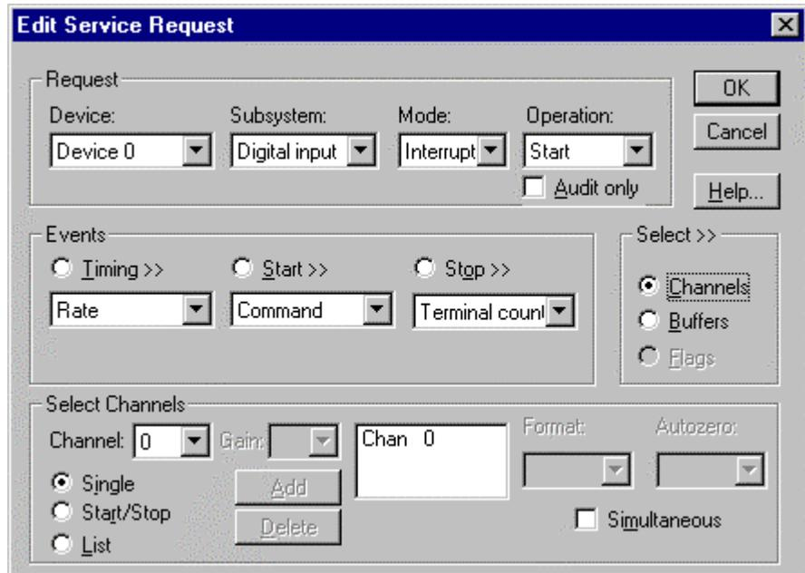
*How to set up the KPCI-PIO to read from a single channel*
