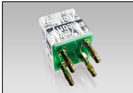
Model 8620 Four-Wire DMM Shorting Plug: Provides a low resistance 4-wire short to both observe and cancel DMM offset resistances and voltages to improve measurement accuracies.
