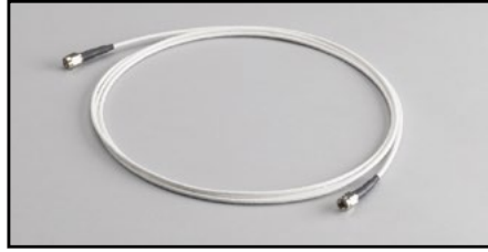
CA-404B: 2m (6.5 ft) RG188 coax cable terminated with an SMA male plug on each end, 50Ω impedance.
