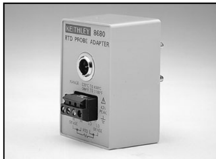
Model 8680 RTD Probe Adapter: Provides a means of connecting RTD probes terminated in either a 4-wire instrumentation connector or bare wires to safety input jacks on a 0.5 inch spacing.
