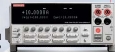
First one-kilowatt pulsed SMU instrument (Model 2430)
