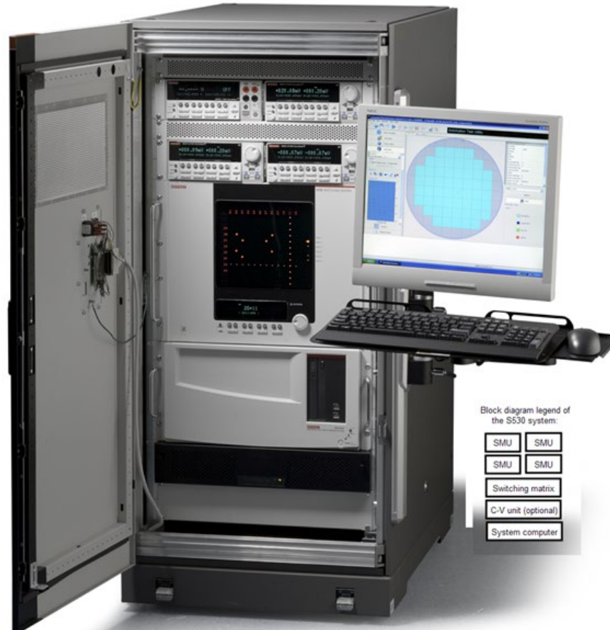
Figure 984: Example HV system configuration
