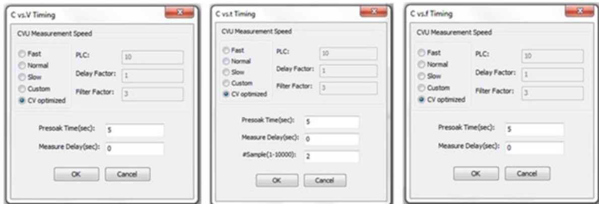
Figure 685: C vs. V, C vs. t, and C vs. f Timing dialog boxes
