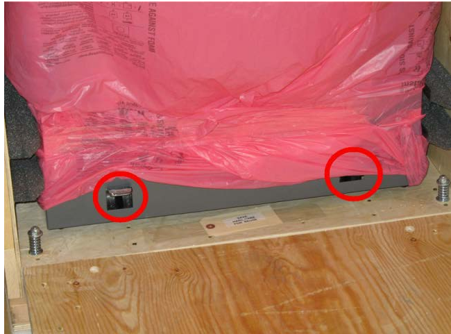
Figure 14: Cabinet caster locks moved up
