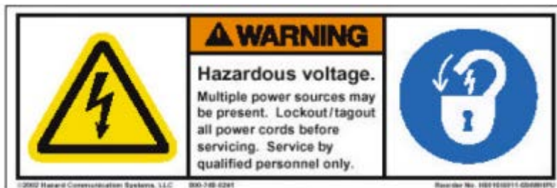
Figure 22: Hazardous warning label
