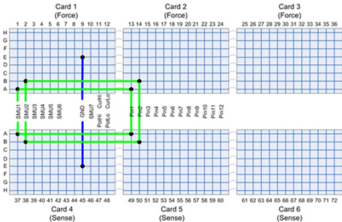
Note that the pin-guard test is similar to the pathway shorts test where a quasi-static, SMU-based capacitance measurement is used to test for guard-to-ground shorts. The maximum capacitance value is 150 pF.
