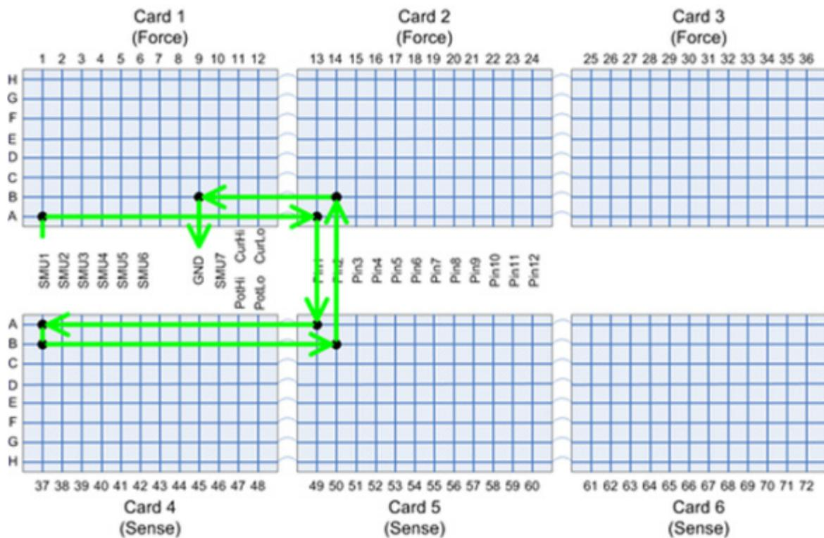
The matrix connections used to validate the isolation relays for pathway A and B between cards 5 and 6 are shown in the next figure.
