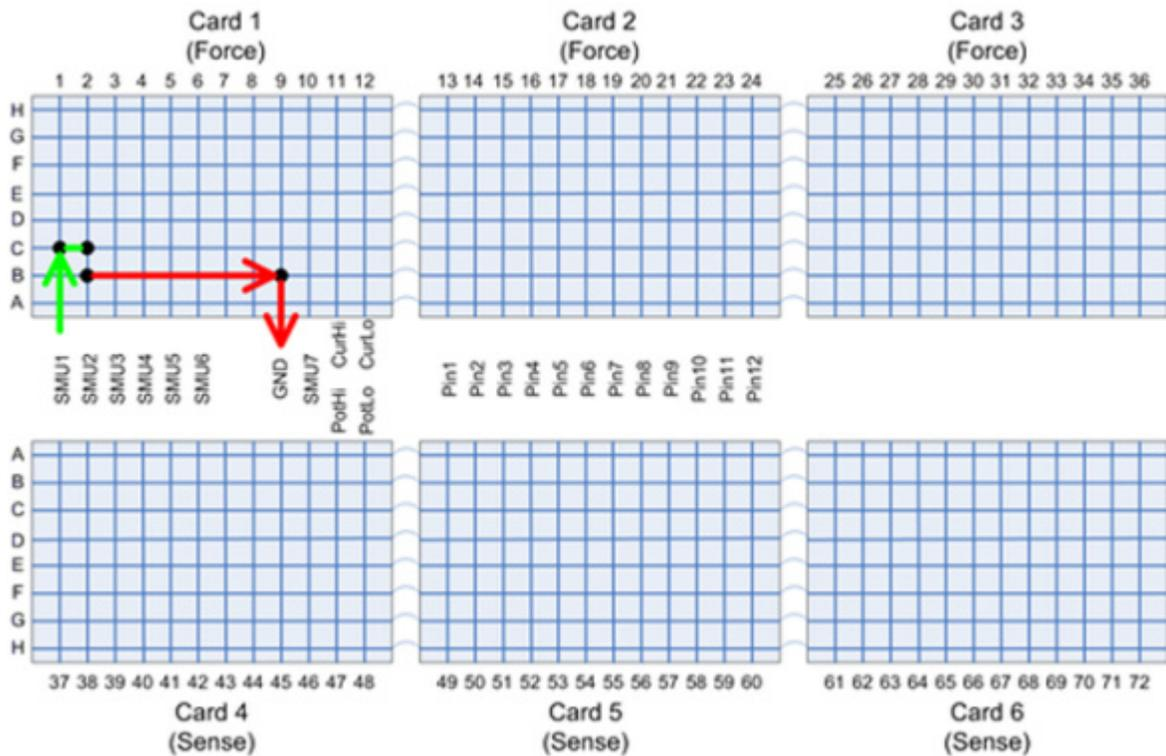
The next figure shows the matrix connections used to validate the column isolation relay for column 2 on card 2.
