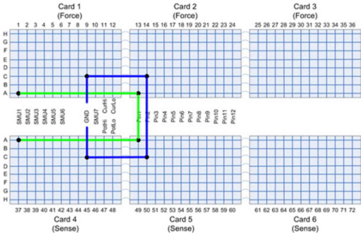
The next figure shows SMU1 and Pin12 connected together during the Kelvin-pin detection. The blue pathway shows Pin1 connected to GND to complete the lo/sense-lo portion of the Kelvin connection. In this example, matrix pathway 'C' is being tested for Kelvin operation and matrix pathway 'E' is used for the GND connection.
