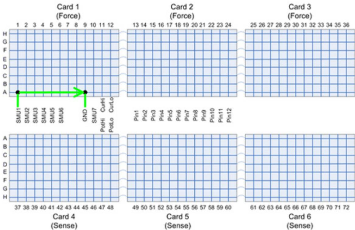
Now that you know that card 1 pathways are good, you can test the card 1 and card 2 connections, and then the card 1 to card 3 connections. You will need to test both combinations in order to determine if card 1, card 2, or card 3 has any failures since we cannot test card 1 directly.
