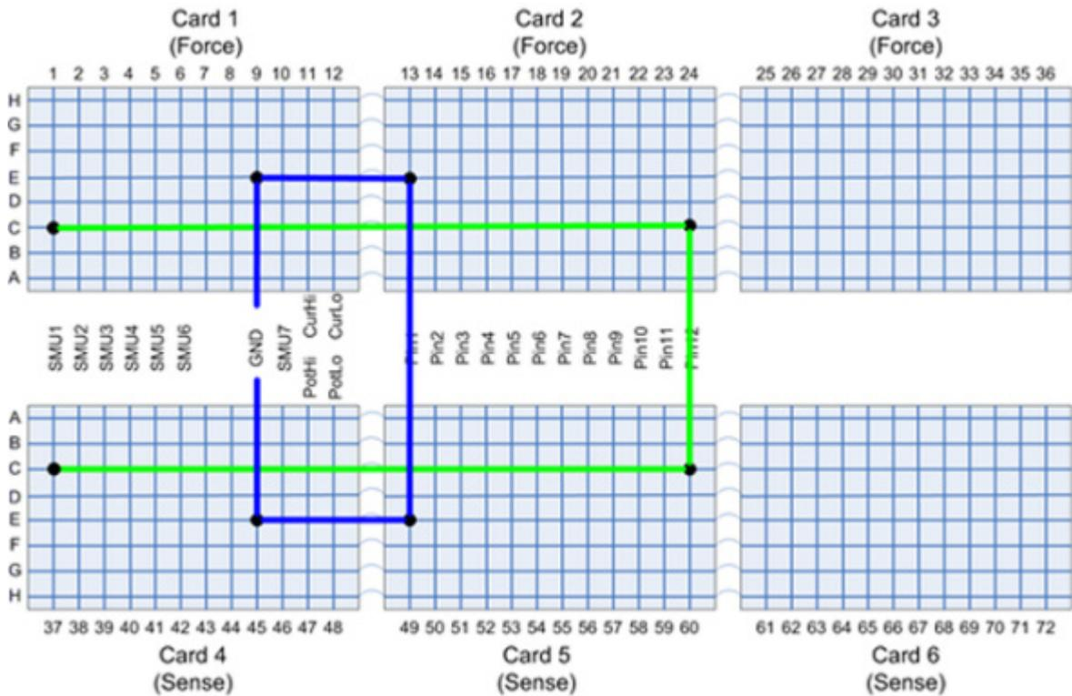
This Kelvin pin-connection test can be individually run to validate connections from the system to the probe card, which is useful after a probe card change or re-cabling. See the [Matrix tab](#) for information on how to configure the diagnostics software to run this test.
