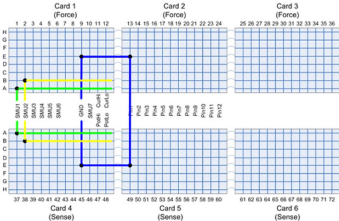
For the second part of the matrix leakage test, a quasi-static capacitance measurement, requiring one SMU, is used to test for potential shorts to the guard signal.
