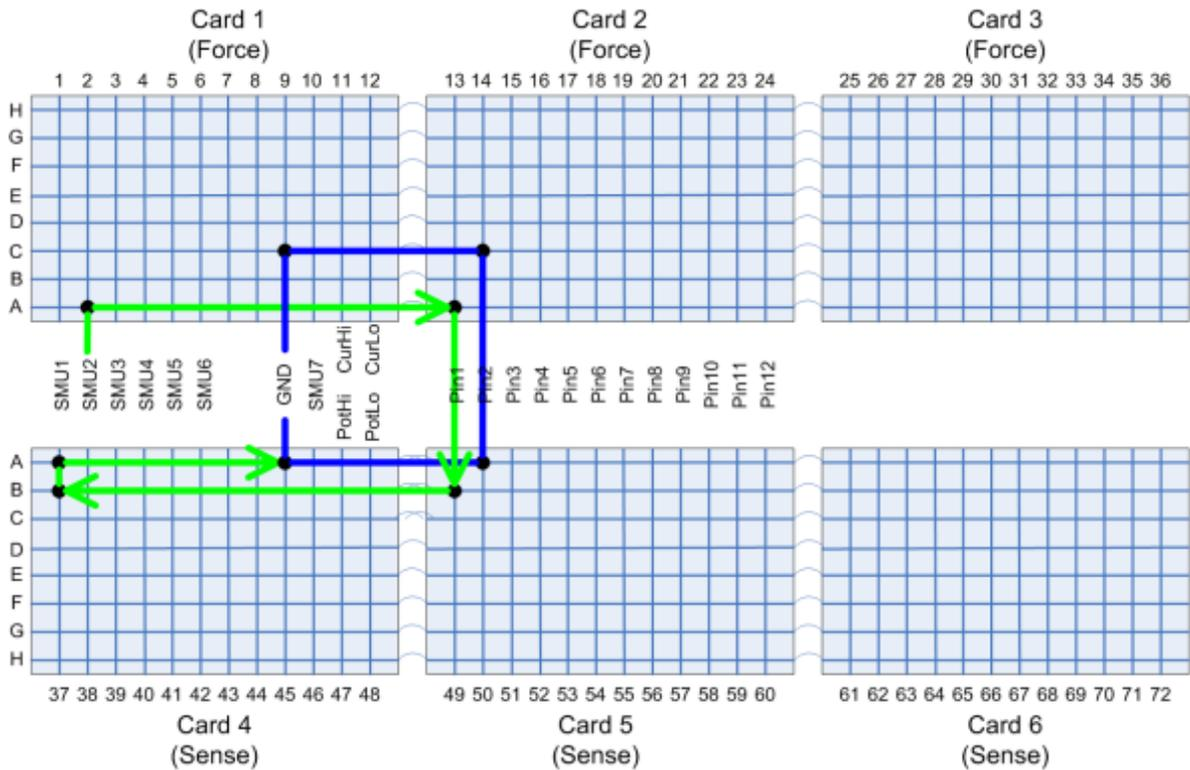
**Figure 15: Sense-side column isolation relay (pre-test pathway C)**
