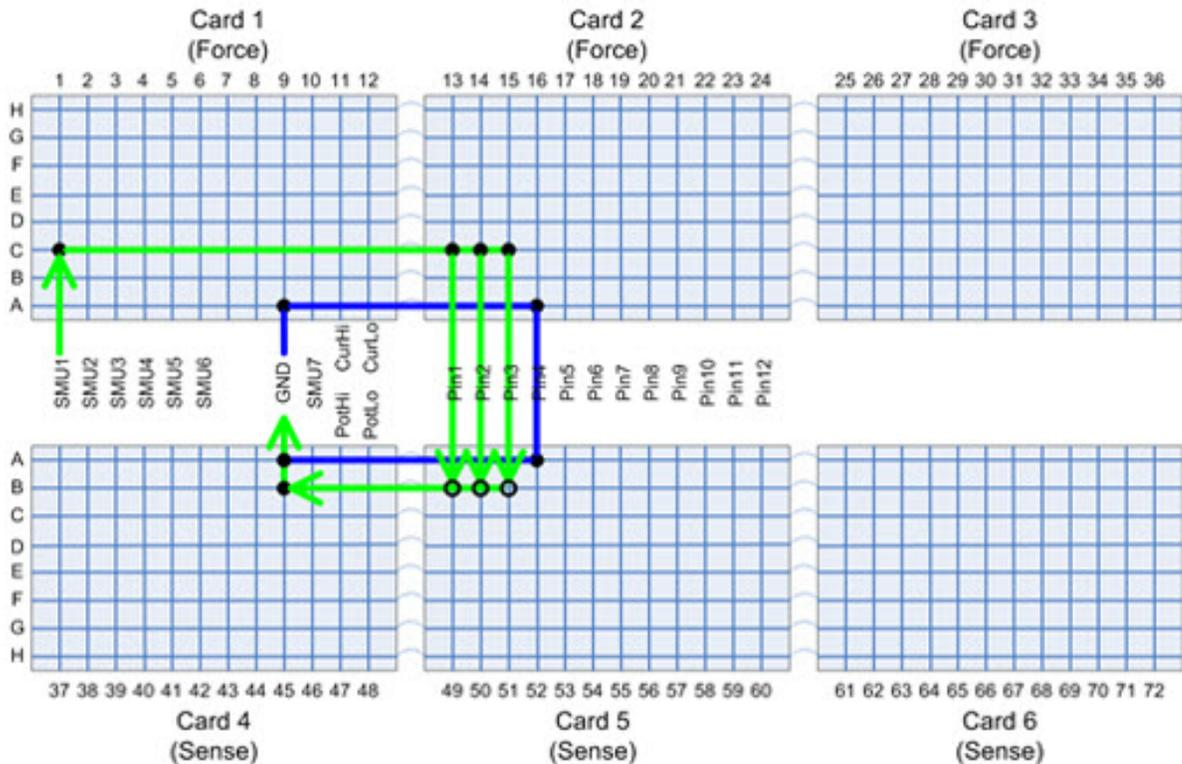
The relays on pathway B on card 5 will be closed and opened, one at a time, and current flow will be measured by the SMU.
