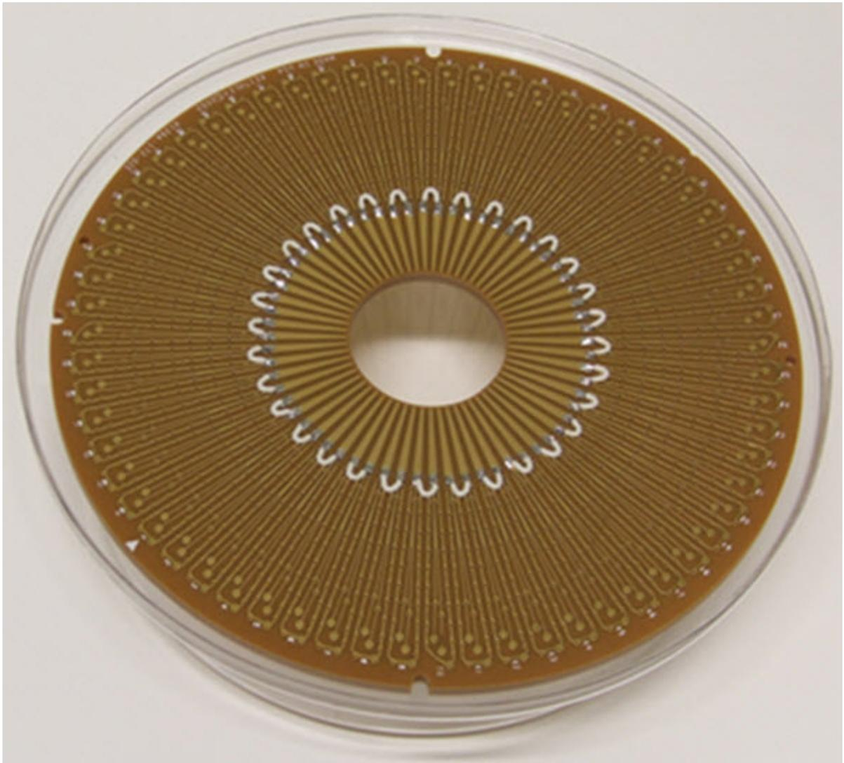
The following blank probe card figure is included so that you can easily see the difference between this card and the verification probe card. Note that the number and configuration of jumpers (white wires in previous figure) on the verification probe card are determined by the system configuration.
