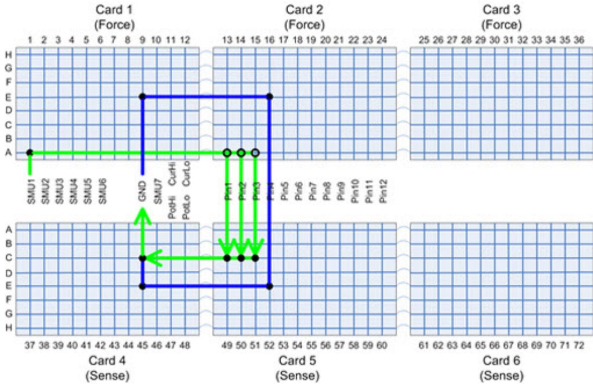
Pins 1 through 3 on the sense card are tested with pin 4 being used for the GND connection. Each of the three relays on columns 13, 14, and 15 will be closed and opened, one at a time, to test the isolation relays on the sense card.
