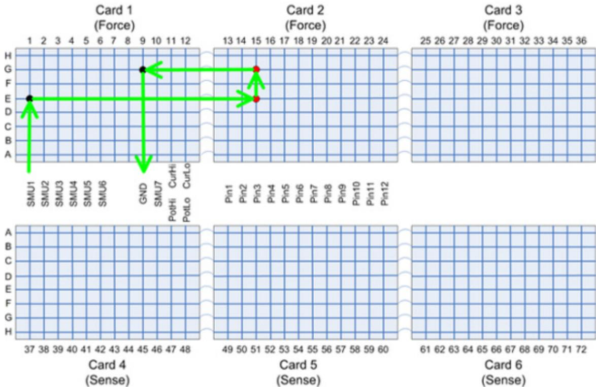
**Model 7072-HVD matrix card discharge circuit test**
