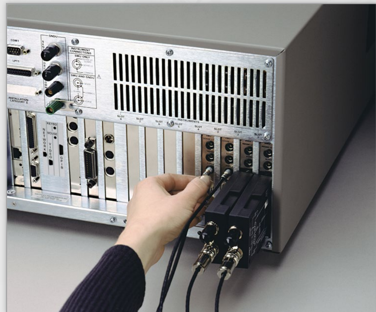
The Model 4200-SCS's DC PreAmps can be mounted on the back of the parameter analyzer or on the probe station. By reducing the signal path between the DUT and the PreAmp, the Model 4200-SCS can reduce cable effects like parasitic capacitance and leakage currents, which provides for more accurate low-level measurements.
