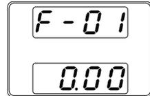
3. Rotate the Voltage knob to change the F setting to F-03 (V-I Mode Slew Rate Select).
