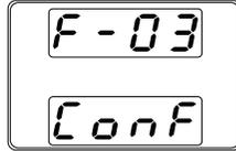
6. If CV Slew Rate Priority was chosen as the operating mode in steps 3~5, set F-04 (Rising Voltage Slew Rate) and F-05 (Falling Voltage Slew Rate) and save.
