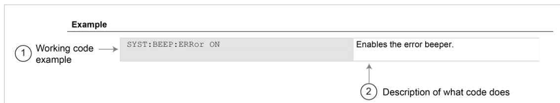
Figure 103: SCPI command description example
