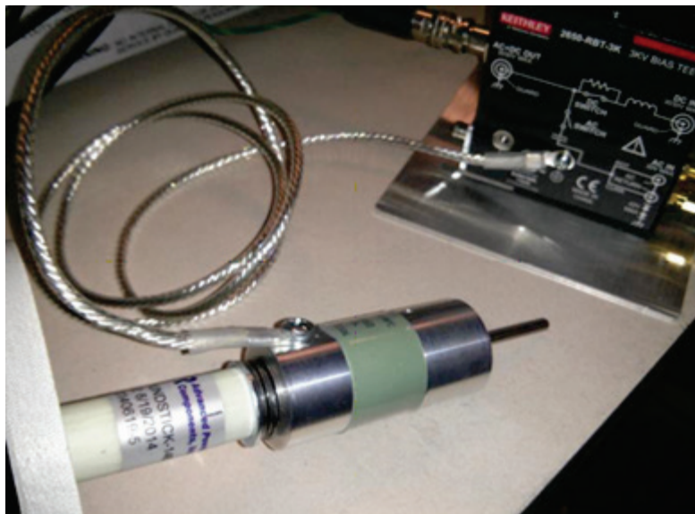
Figure 77: 8020-DP connected to bias tee protective earth screw
