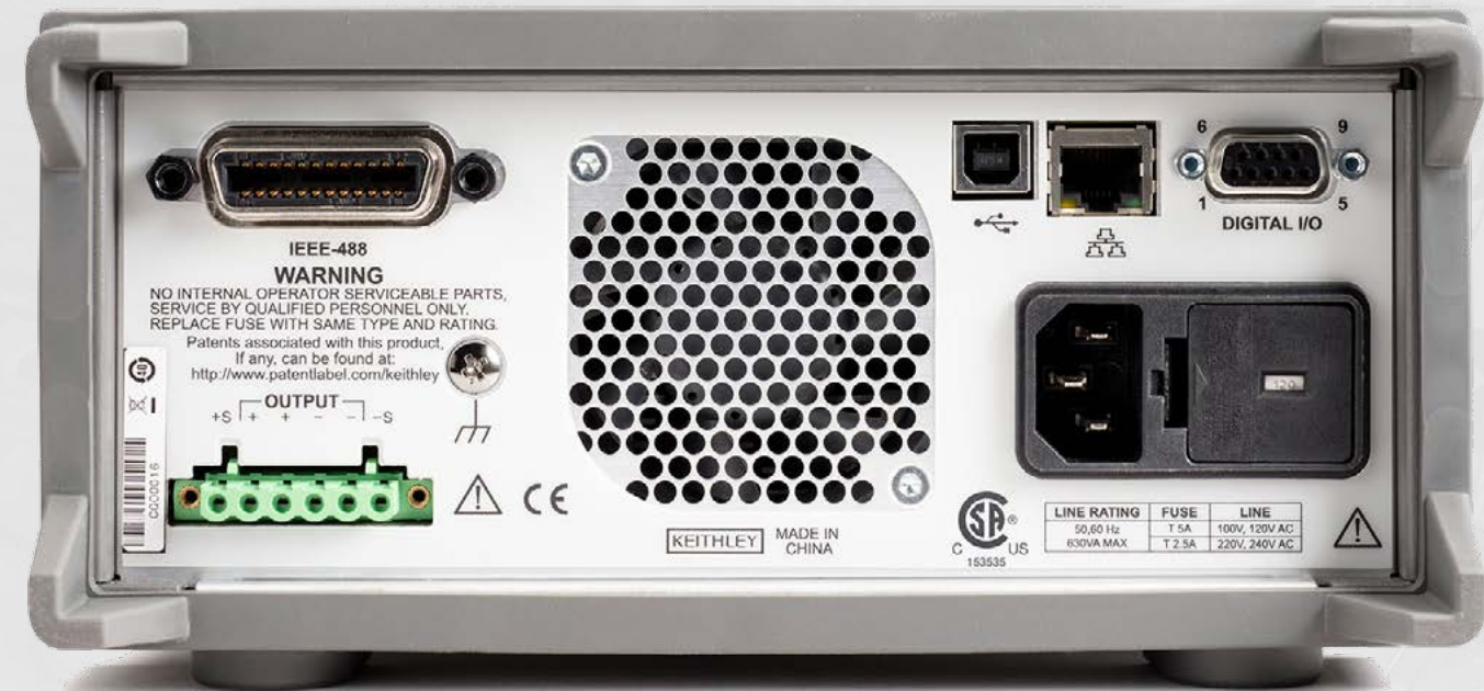
Series 2280S rear panel showing the rear output connector with remote sense inputs, digital I/O, and the GPIB, USB, and LAN interfaces.
