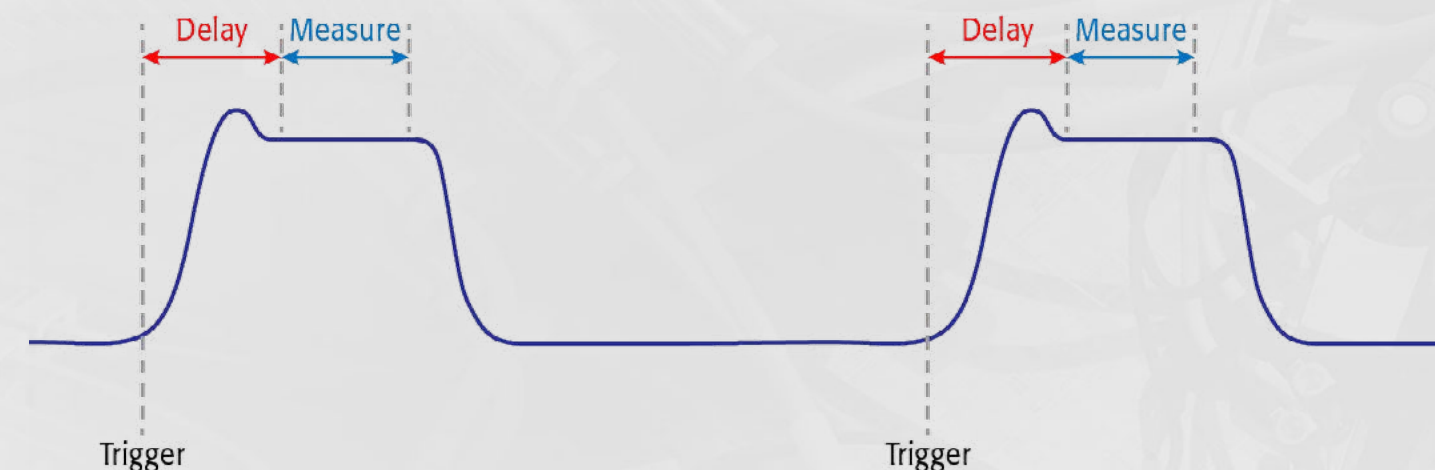
Make time-critical measurements on fast-changing or pulse-like loads. An external trigger initiates the acquisition. Programmable delay and measure times enable measurements at a specific time on the load current pulse.
