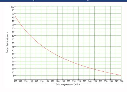
To maintain safe start-up  $\mathbf{R}_{\scriptscriptstyle{M}}$  must not exceed 20  $\Omega$  during fault condition.
